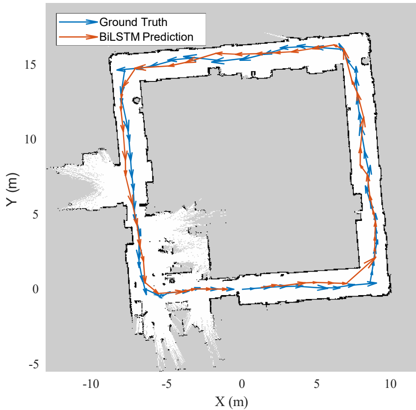
Figure 3: BiLSTM’s predicted locations vs ground truth at EOW 3rd floor (Dataset A: Wi-Fi+BLE).
